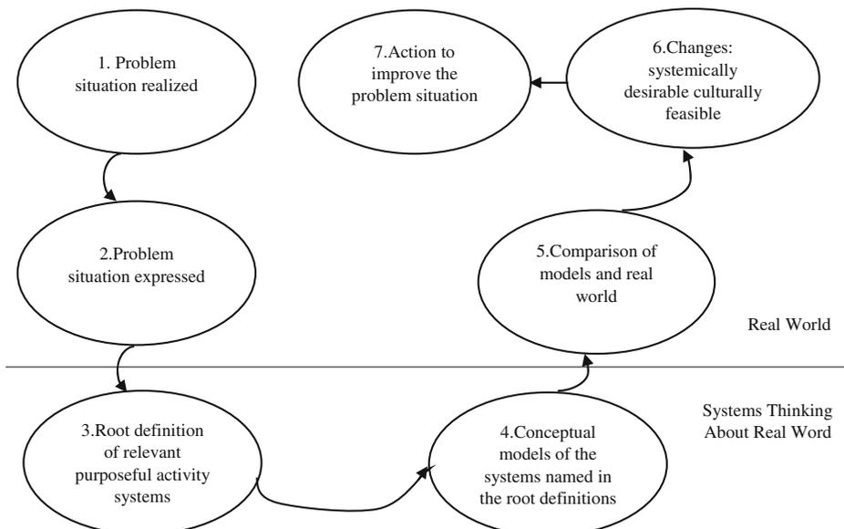
**Fig. 3** The conventional seven-stage model of SSM (Checkland and Scholes 1990)
